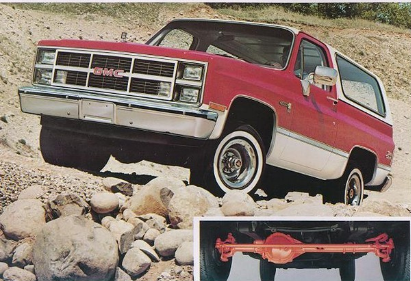
Jimmy's front suspension includes leaf springs and stabilizer bar.
